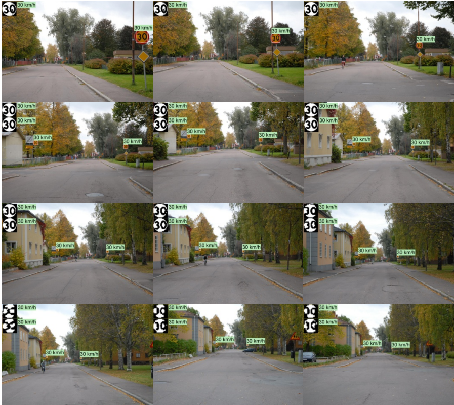
Figure 9. Classification of speed limit traffic sign on different distances. Top Left: 10 m distance, Bottom Right: 120 m distance. Images are taken in 10 m step.
