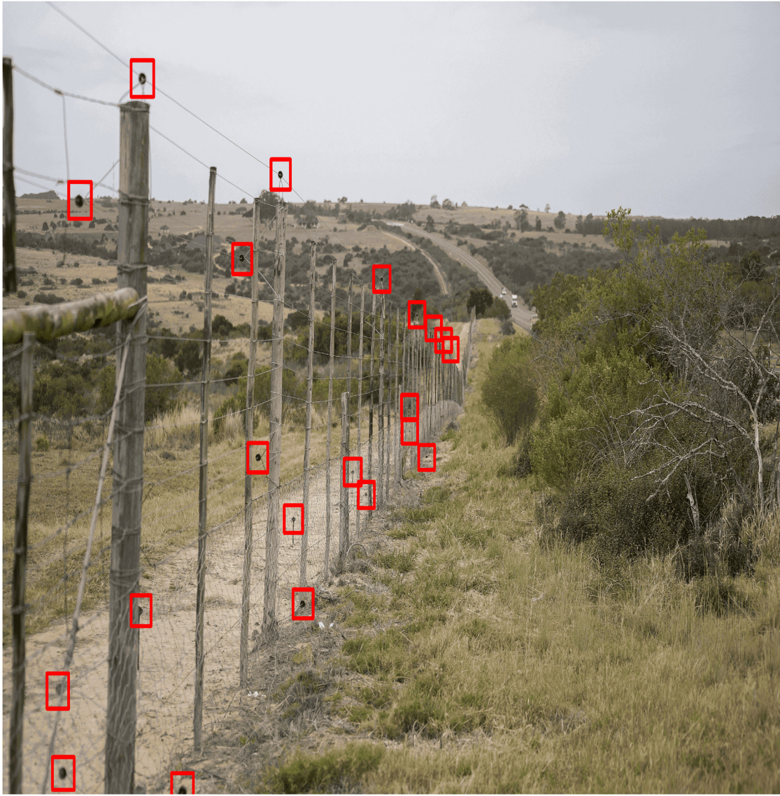
Figure 14: Detected insulators on wildlife electric fence at Amakhala private game reserve from the still dataset [50].
