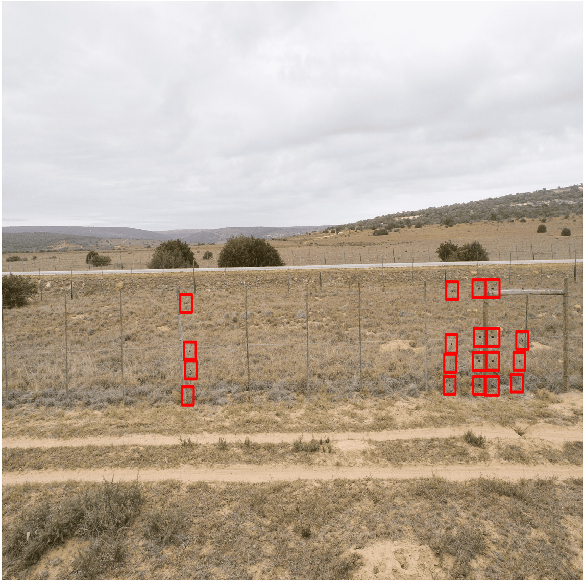
Figure 13: Detected insulators on wildlife electric fence at Amakhala private game reserve from the aerial dataset [50].
