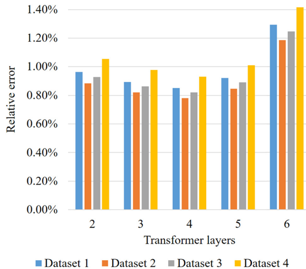
Figure 10: The influence of different transformer layers on fault location results. Source: Created by the authors.
