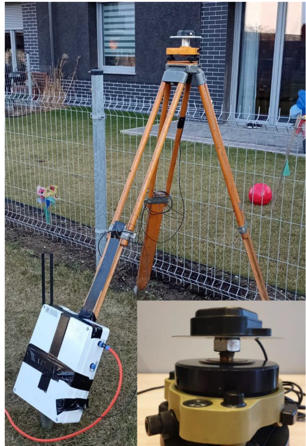
Figure 14: The method of mounting the u-blox patch antenna on the tribrach.
