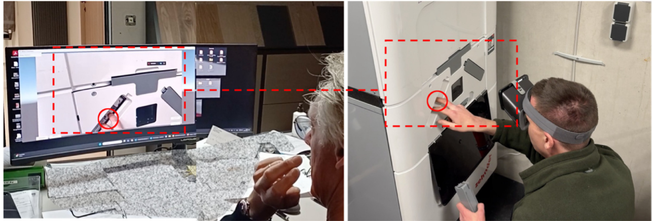
Figure 1: Our AR HMD-based remote system application in field use. Left: A consultant discusses the maintenance of a heating system remotely. The red circles are the visual cues placed by the remote worker. Right: An on-site employee discusses problems and answers questions regarding which steps have already been taken.
