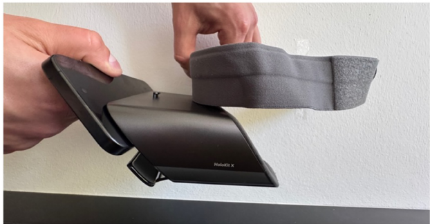
Figure 2: The Holokit mount with an inserted smartphone (iPhone 15).
