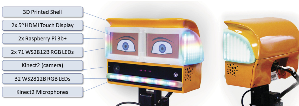
Figure 3: The robot's head with its components.
