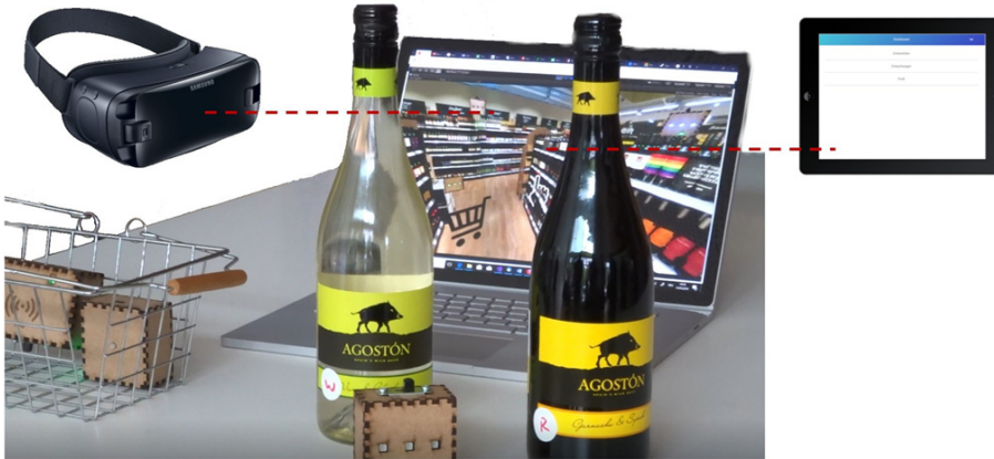
Figure 2: Virtual AR-Prototype on Gear VR (ExProtoVAR) coupled with prototype for IoT devices (C-Blocks) and integrated web-app to assist users finding the correct wine.
