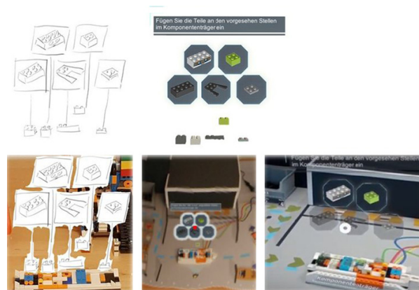
Figure 6: Design of placing instruction: Top row: 2D sketches and screen designs; Lower row: Simulated appearances with ExProtoVAR (LL, LC) and final visualization in the MS HoloLens (LR).
