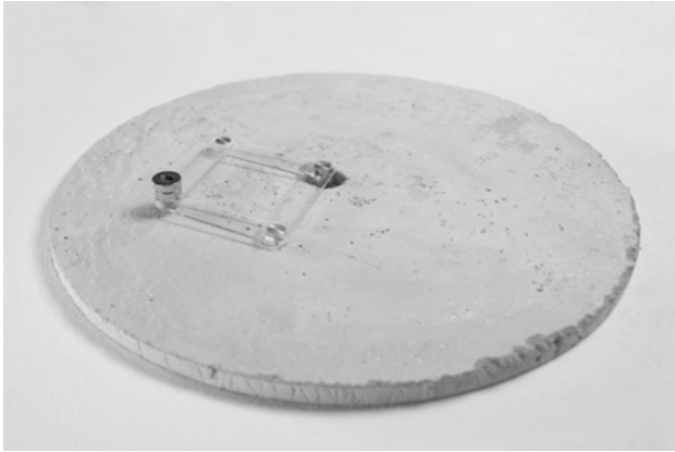
Figure 4: Concrete Data: a stone-based data logger.
