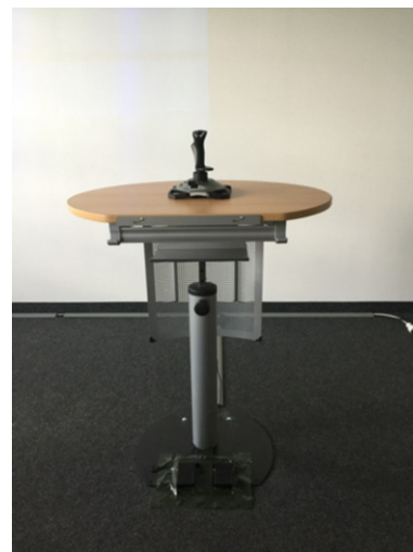
Figure 3: Photograph of the standing desk with the joystick and the double foot pedal.
