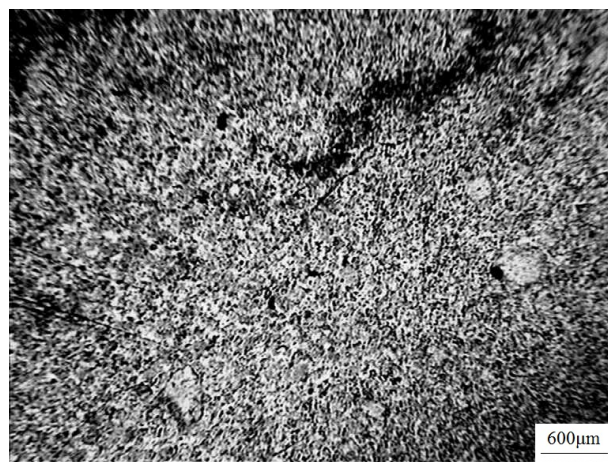
Figure 4. Microstructure of the specimen quenched with 9 Hz, 500 V, 9 min and 1200 \mu\text{F} \times 50 .
