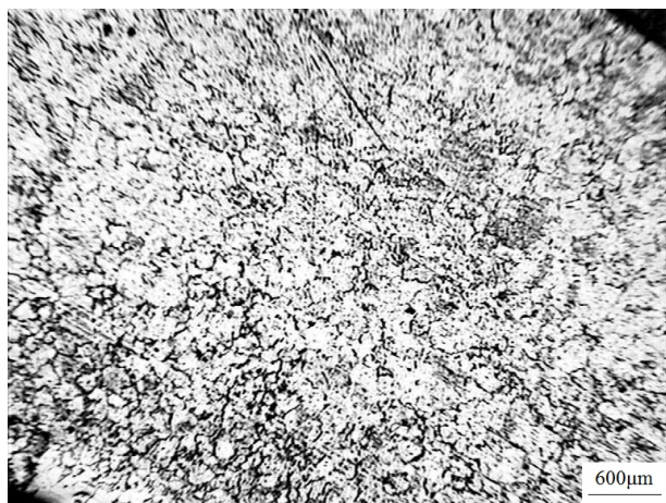
Figure 2. Microstructure of the specimen quenched without the PEF treatment \times 50 .
