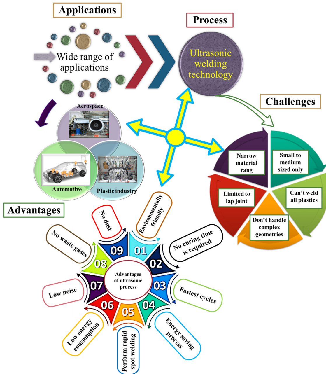
Figure 2: The detailed flow chart for applications, advantages, and challenges of the ultrasonic welding technique [16,38].
