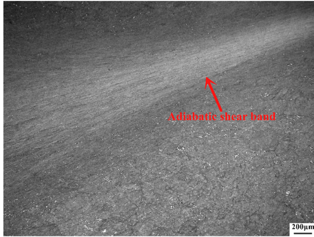
Figure 14: Adiabatic shear band observed at high strain rate of 10 \text{ s}^{-1} .
