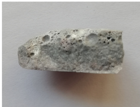
Figure 1: Macro morphology of slag after reaction.
