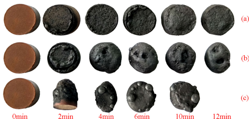
Figure 3: The melting and separation of red mud at different times and temperatures: (a) 1,350°C, (b) 1,400°C, and (c) 1,450°C.
