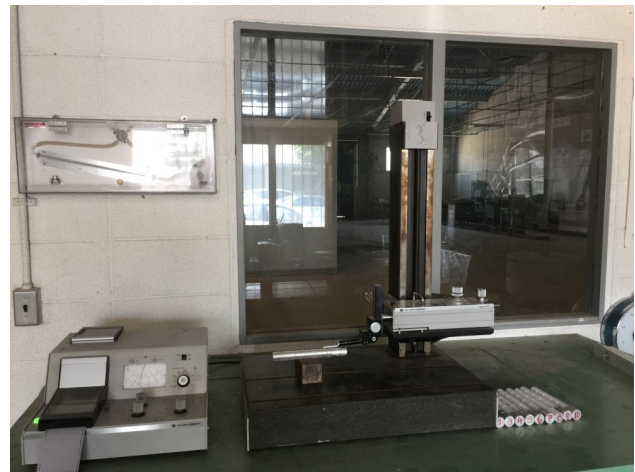
Figure 4: A TAYLOR-HOBSON (10) surface roughness device.
