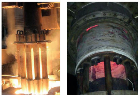
Figure 25: Electroslag remelting hollow ingot in plant.
