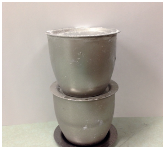
Figure 3: Ni crucibles after 1,000 h corrosion test.
