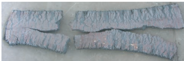
Fig. 5: The cracked flat ingot in hot rolling process
