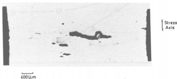
Fig. 4. (b) Void profile at failure in 30 min. compressive dwell test (1CrMoV steel, 565°C /11/)
