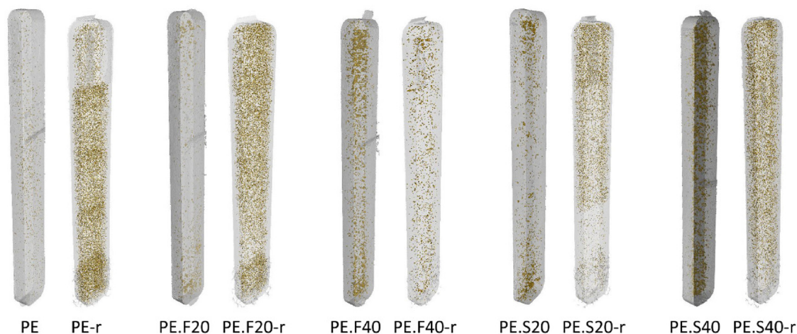
Figure 15: 3D computed tomography images presenting pores distribution.
