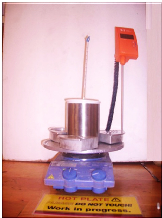
Figure 4: A laboratory-scale prototype of a Mozafari vessel, made of pharmaceutical-grade stainless steel, with a volume of 1Lt.
