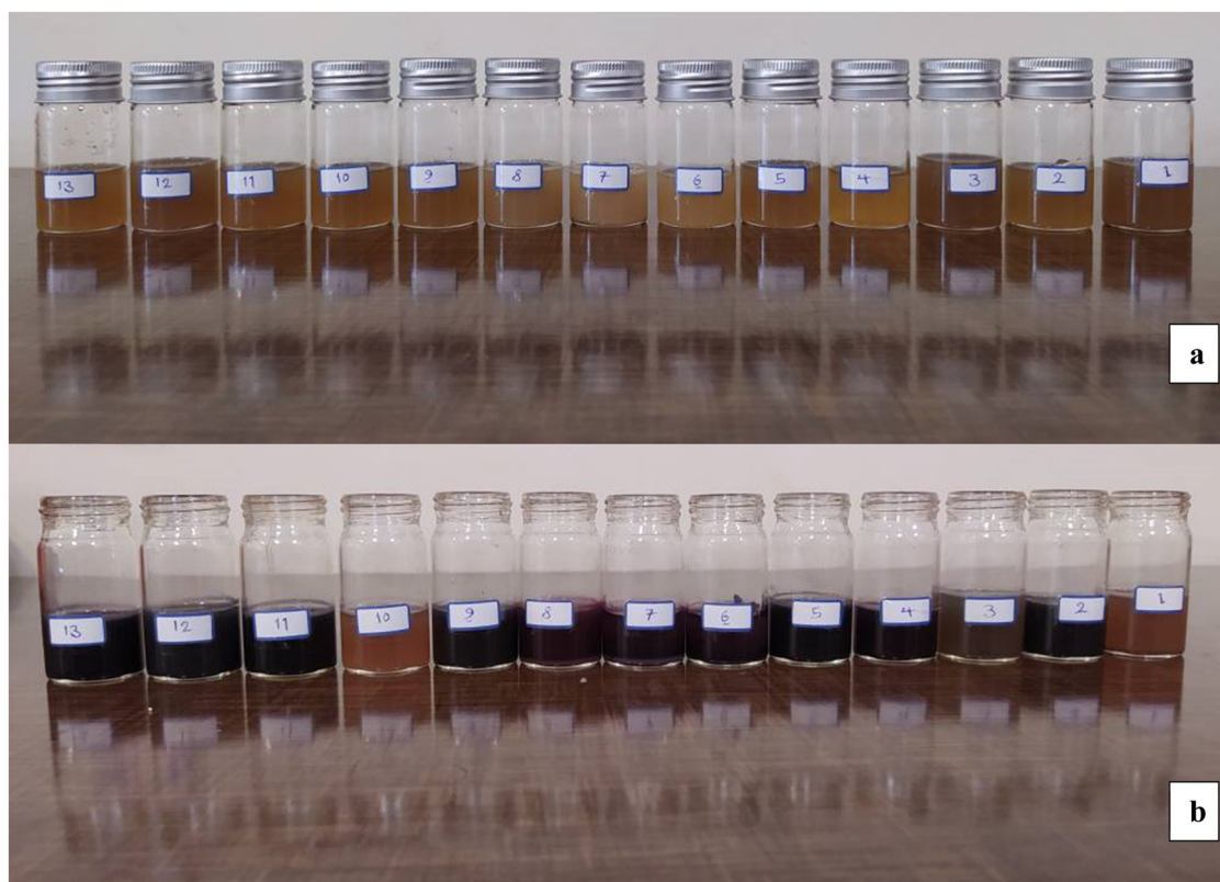
Figure 7: Appearance and color of the mixture solution before (a) and after (b) formation of the Au NPs via UV radiation.
