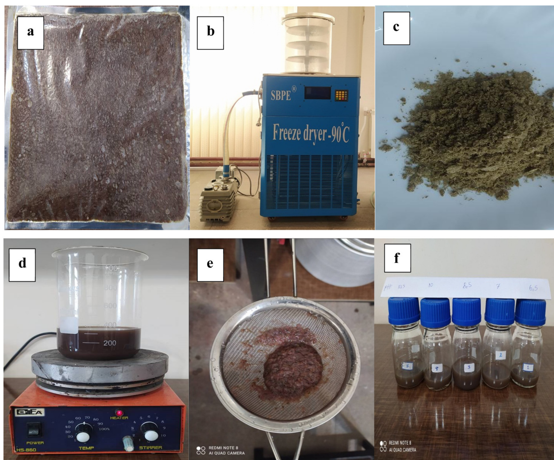
Figure 1: Schematic of the preparation of A. urumiana extract: frozen A. urumiana (a), freeze dryer (b), A. urumiana powder (c), dissolution of powder (d), filtration (e), and pH adjustment (f).
