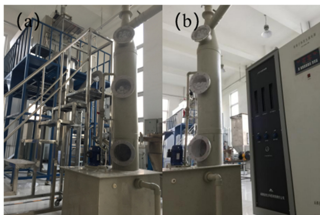
Figure 2: Picture of off-gas treatment unit connected with (a) RF and (b) DC plasma reactor.
