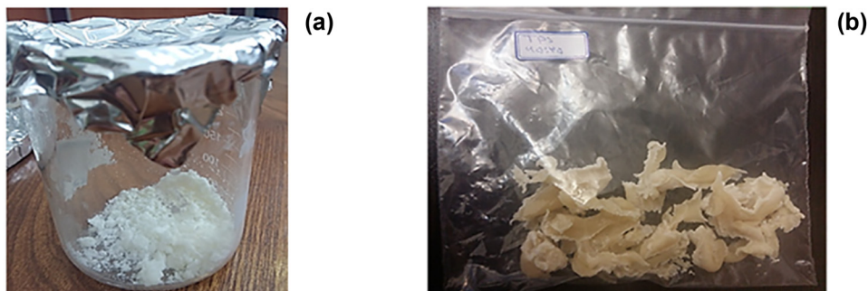
Figure 2: Mixture of starch and glycerol (a) and thermoplastic starch (b).
