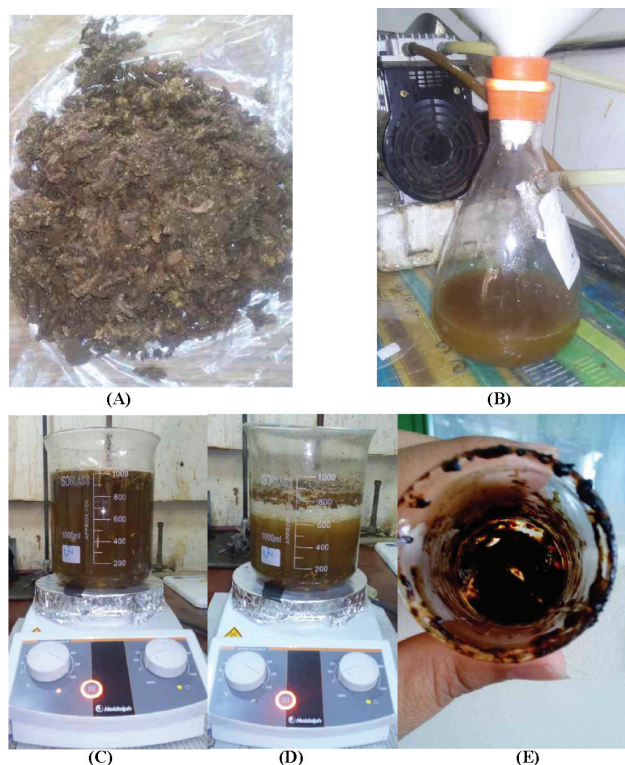
Figure 3: An illustration for different stages of Gypsophila aretioides extraction (a) grated roots, (b) aqueous extract, (c) clarified extract, (d) boiling extract and (e) dried extract.
