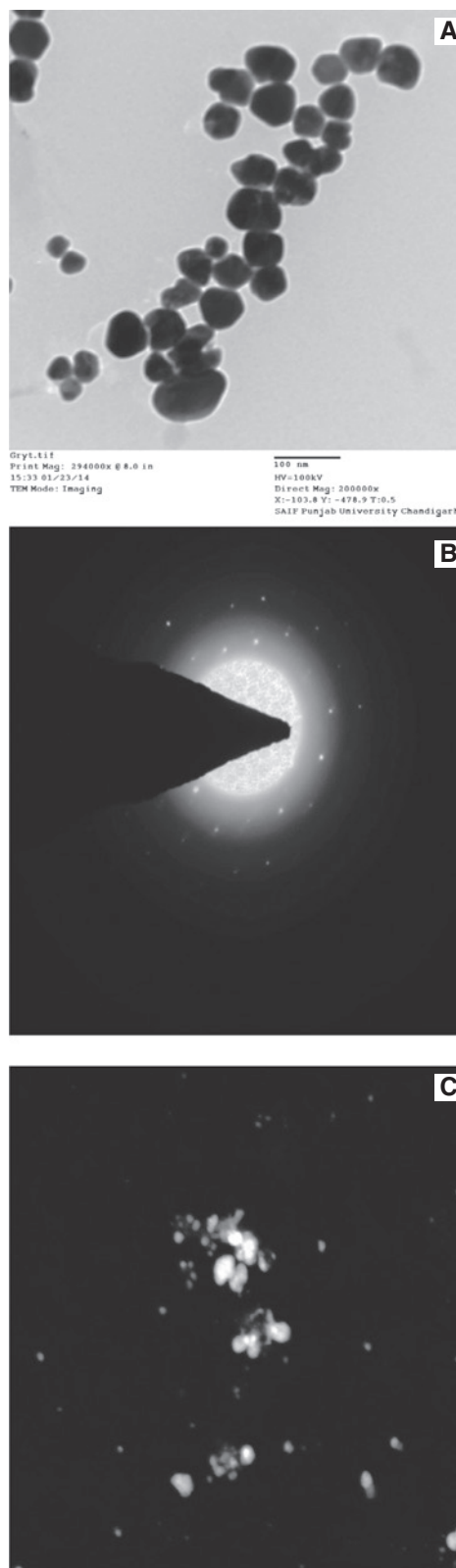
Figure 4: The TEM images of the Ag nanoparticles synthesized using the cellular extract of Penicillium oxalicum GRS-1. (A) TEM image of Ag nanoparticles at a scale of 100 nm. (B) Selected area electron diffraction pattern (SAED) of Ag nanoparticles. (C) High Resolution TEM image of biologically synthesized Ag nanoparticles.
