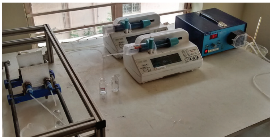
Figure 1: Experimental set-up for synthesis of performic acid in advanced-flow reactor (AFR) – two modules.
