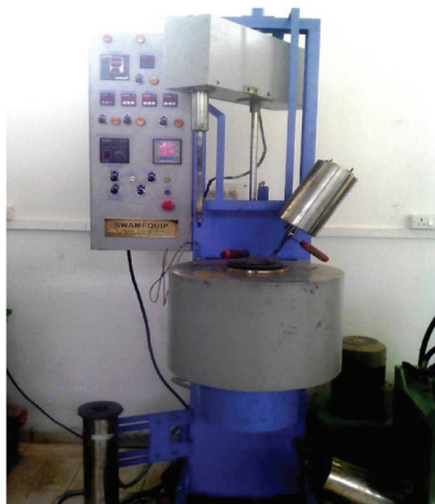
Figure 2: Bottom pouring stir casting apparatus.
