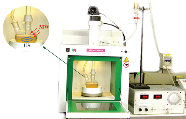
Figure 1: Set up of simultaneous ultrasound-microwave irradiation apparatus.
