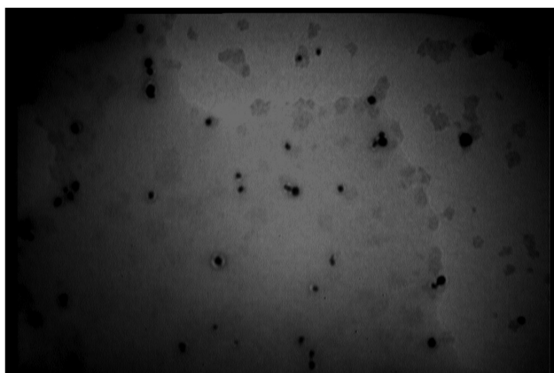
Figure 5 Transmission electron microscopy (TEM) micrograph recorded from a drop-coated film of an aqueous solution of \text{Ag}^+ ions incubated with freshly cultured S. boulardii (after 5 h biotransformation).
