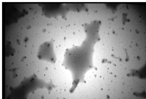
Figure 3 Transmission electron microscopy (TEM) micrograph recorded from a drop-coated film of an aqueous solution of \text{Ag}^+ ions incubated with freshly cultured S. boulardii (after 5 h biotransformation). Magnification is: 5000.
