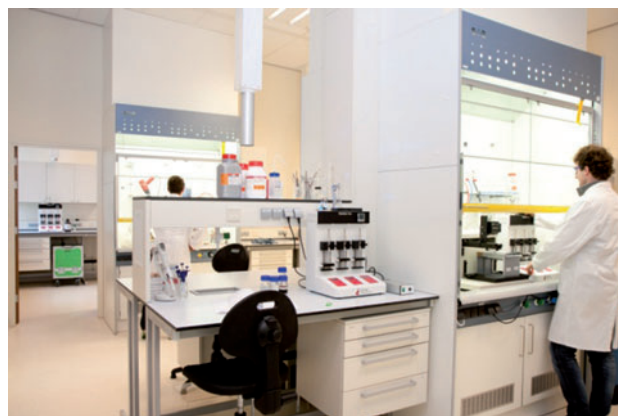
Figure 3 FlowSafe for production and development of PET-tracers in the hospital.
