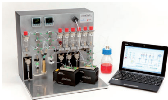
Figure 3 FlowSafe for production and development of PET-tracers in the hospital.
