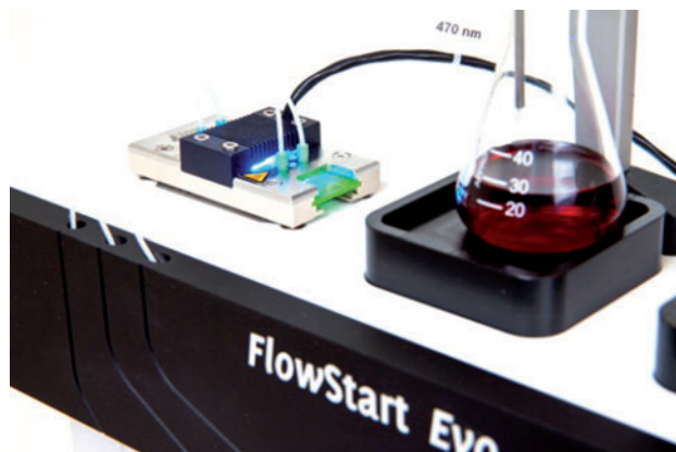
Figure 1 Photochemistry module with the FlowStart Evo.
