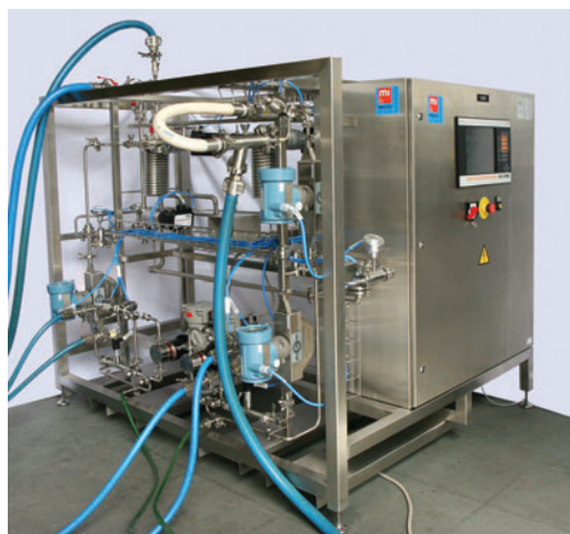
Microinnova unit operation: replacement of one or more individual batch-steps with continuously operated modules.
