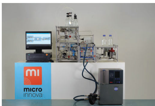
Flow Miniplant: Bench-top pilot plant, plant for development and small-scale production.
