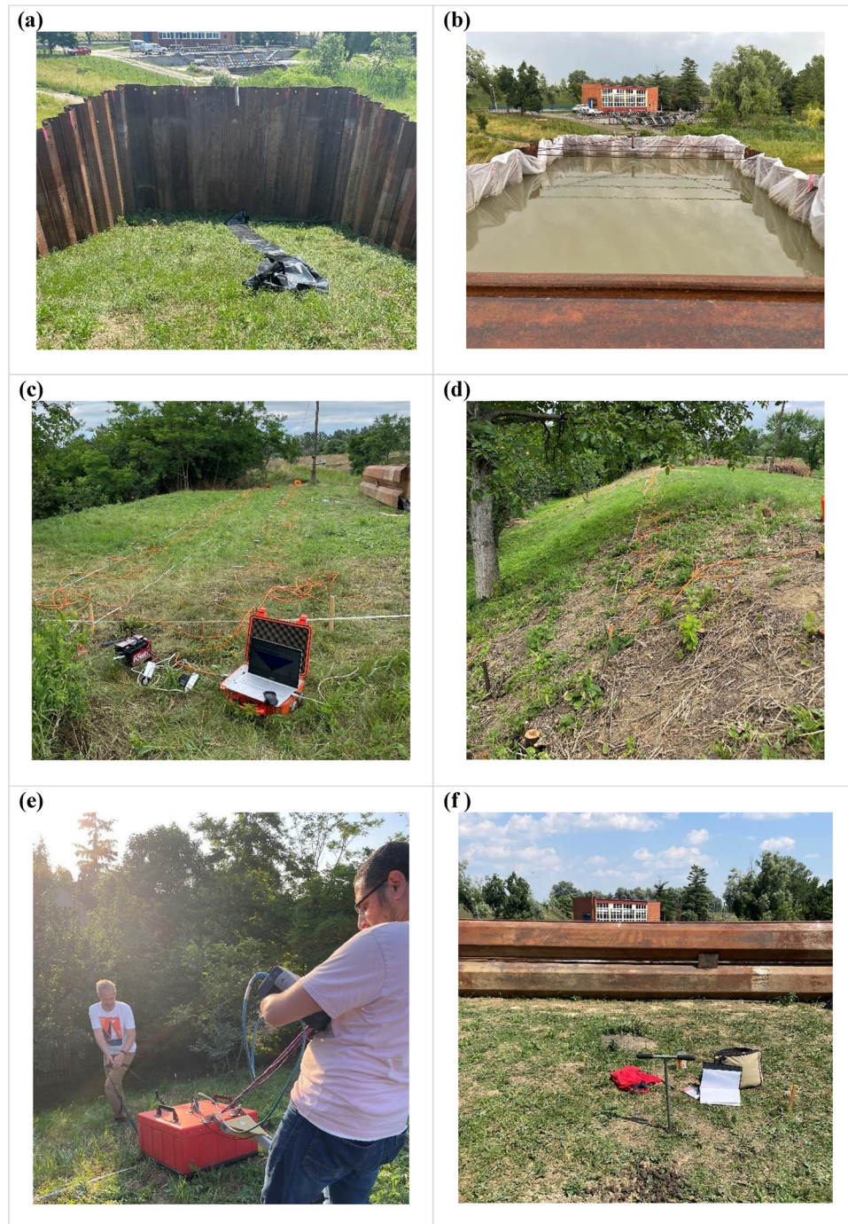
Figure 2: Field photos of the tank (a) before and (b) after filling with water; ERT data acquisition on the (c) levee crown and (d) protected side; (e) GPR data acquisition; and (f) BH drilling.
