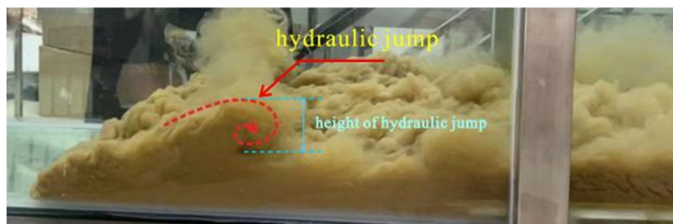
Figure 5: Underwater hydraulic jump phenomenon.
