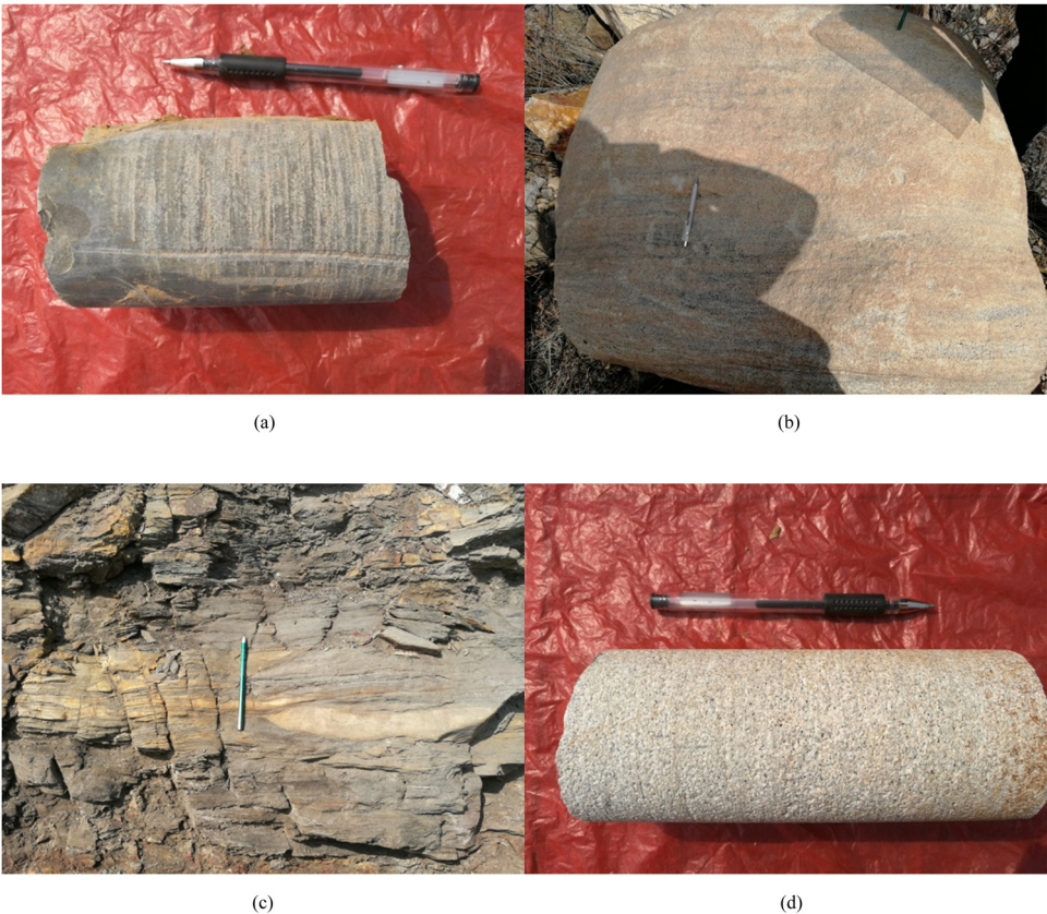
Figure 3: Characteristics of hand specimens from coal measures of the Taiyuan Formation: (a) gray mudstone – siltstone in the Maoergou section, (b) Malan sandstone – fine-grained lithic quartz sandstone, (c) Jinci sandstone – fine-grained quartz sandstone, and (d) Qiaotou sandstone – coarse-grained lithic quartz sandstone.
