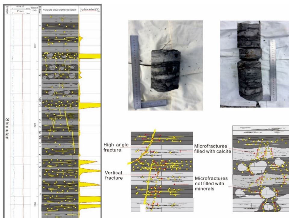
Figure 17: Fractures development pattern of the Shiniulan Formation core samples.
