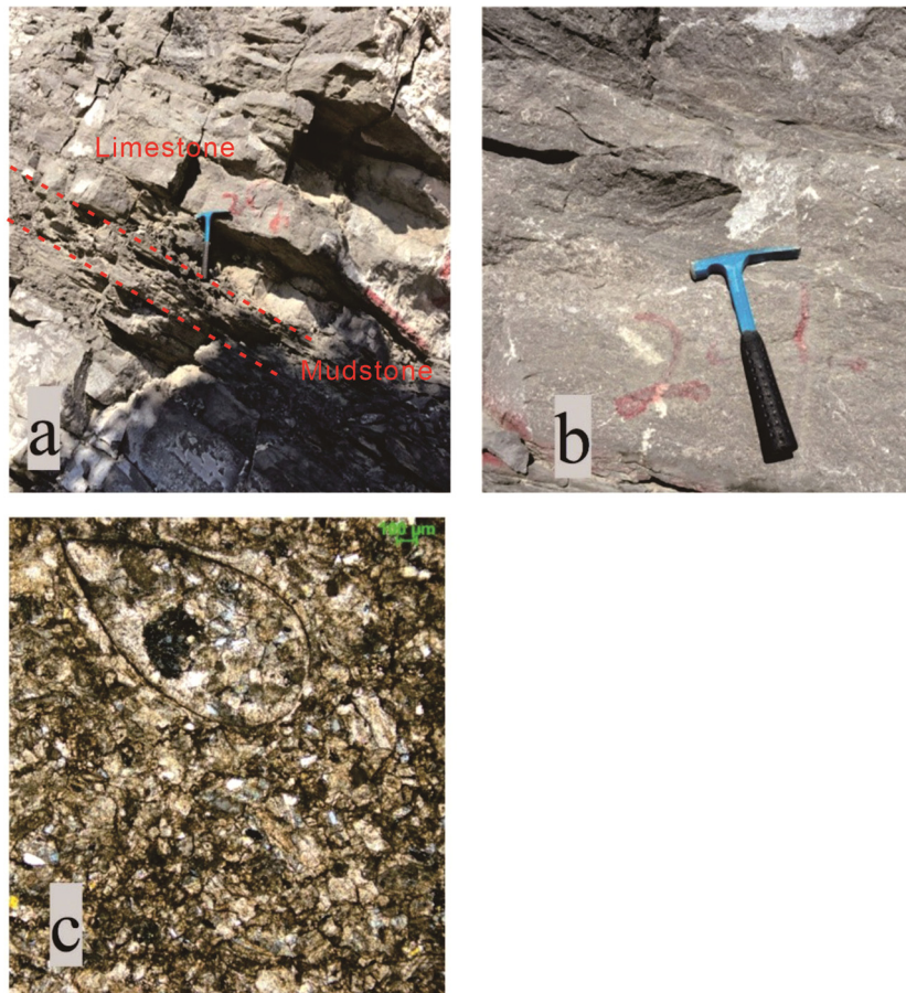
Figure 6: The characteristics of thick limestone and mudstone and thin section of samples observed under microscope. (a) Irregular interbed of thick limestone and mudstone. (b) Thick limestone. (c) The siliceous structure contains siliceous and Bioclastic sparry. The sample is mainly composed of calcite, followed by quartz and other minerals. The stratification can be clearly seen under the microscope.
