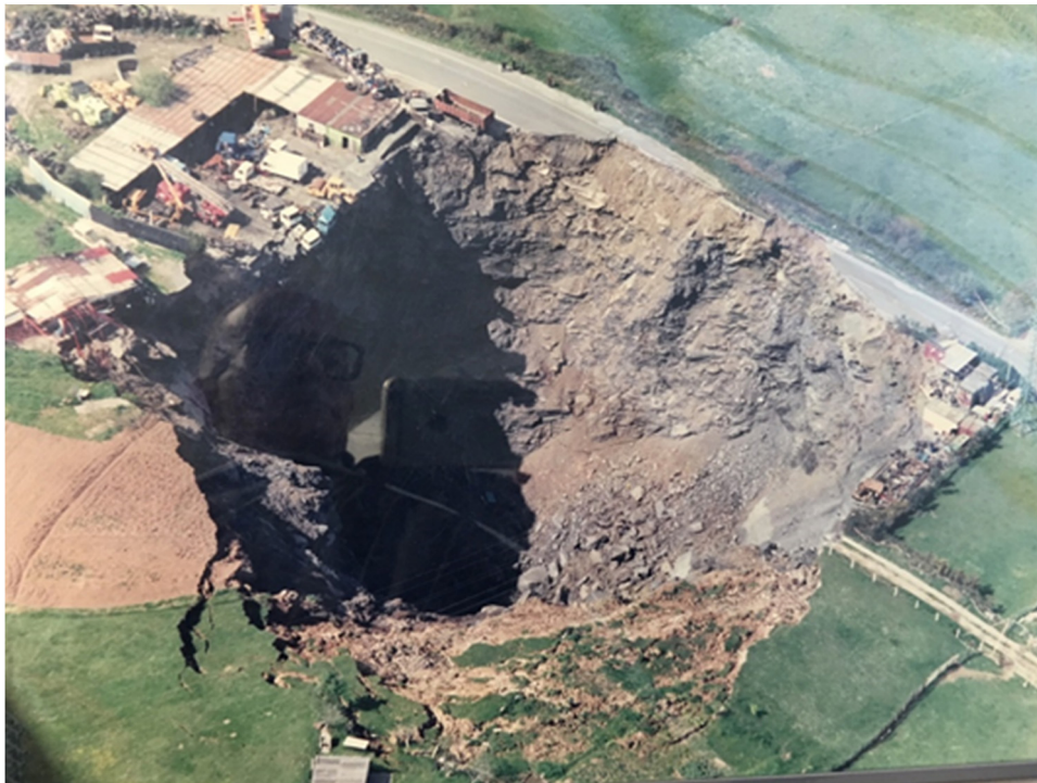
Figure 2: Aerial photograph of the surface crater resulting from the 1999 collapse (image by the authors).
