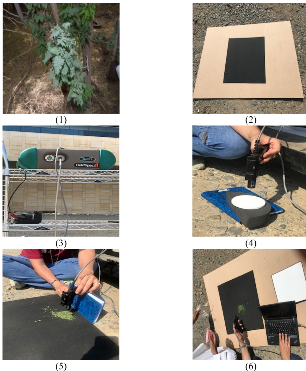
Figure 2: Pictures showing the mechanism of work (1) plant leaves, (2) black plate, (3) spectroscopy, (4) white reflector, (5) measured by pistol, and (6) transfer of data to the laptop.
