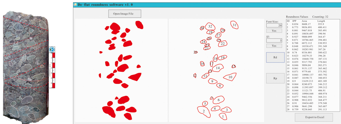
Figure 2: Particle extraction process of core images by the de-flat roundness software, modified from ref. [35].
