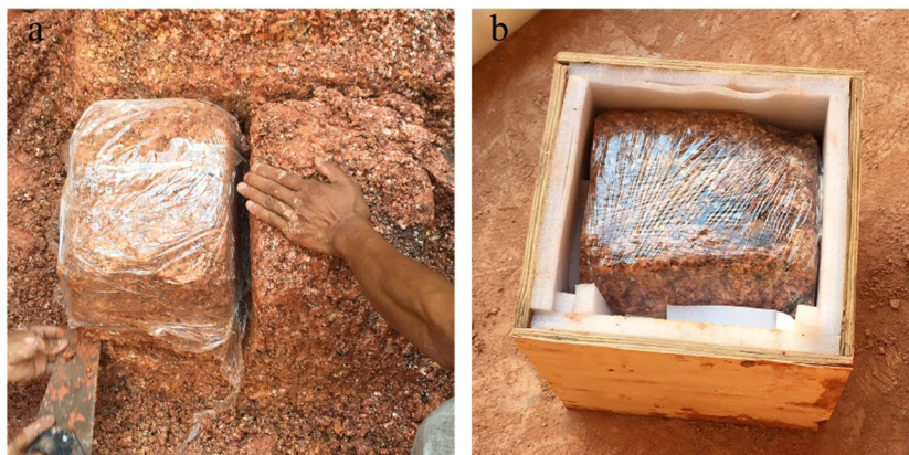
Figure 2: Photos of specimen: (a) cut soil specimen, and (b) specimen packed in the wooden box.
