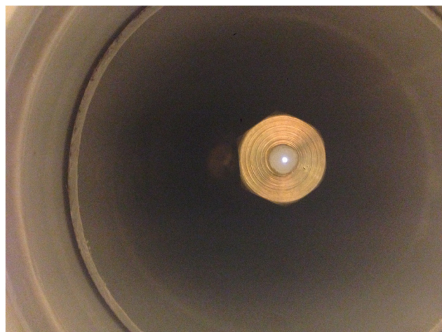
Figure 4: The bottom view of the hanging weight with the glowing core of the optical fibre (own elaboration).
