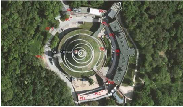
Figure 13: The aerial view of the mound with points of the TLS location.
