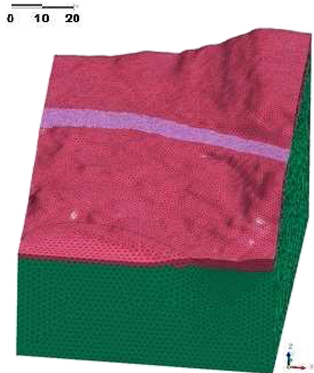
Figure 4: 3-D model of the terrain implemented into the FEM package MIDAS GTS NX.
