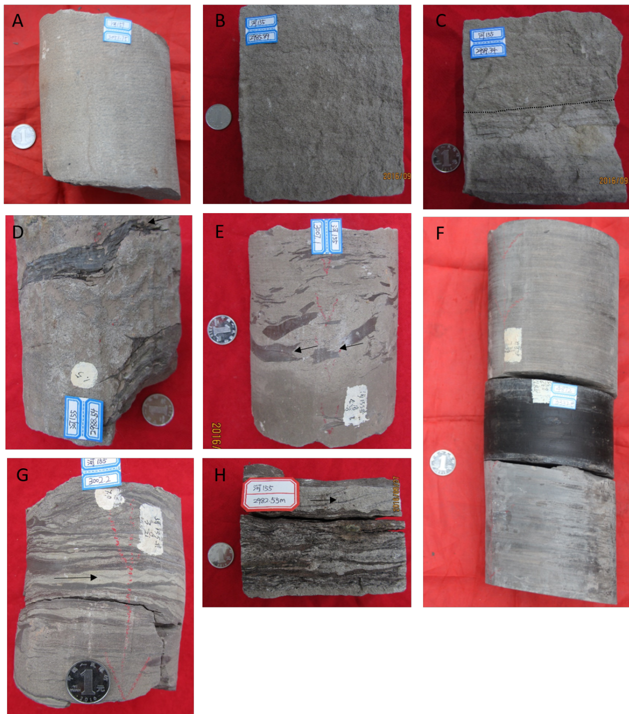
Figure 4: Figure shows different lithofacies with their diagnostic features. (A) and (B) are massive sandstone facies (lithofacies 1); (C) Carbonaceous clast rich sandstone (lithofacies 3) grading into massive sandstone (lithofacies 1); (D) and (E) showing large clasts are floating in muddy sandy matrix, clasts are abraded by surrounding sandy matrix (Black arrows) (lithofacies 2); (F) \Showing parallel lamination, where fine sandstone or siltstone is laminated with gray mud (lithofacies 4); while in the middle is massive dark gray to black hemiplegic mudstone; (G) and (H) inclined imbricated laminae forming duplex-like structures.
