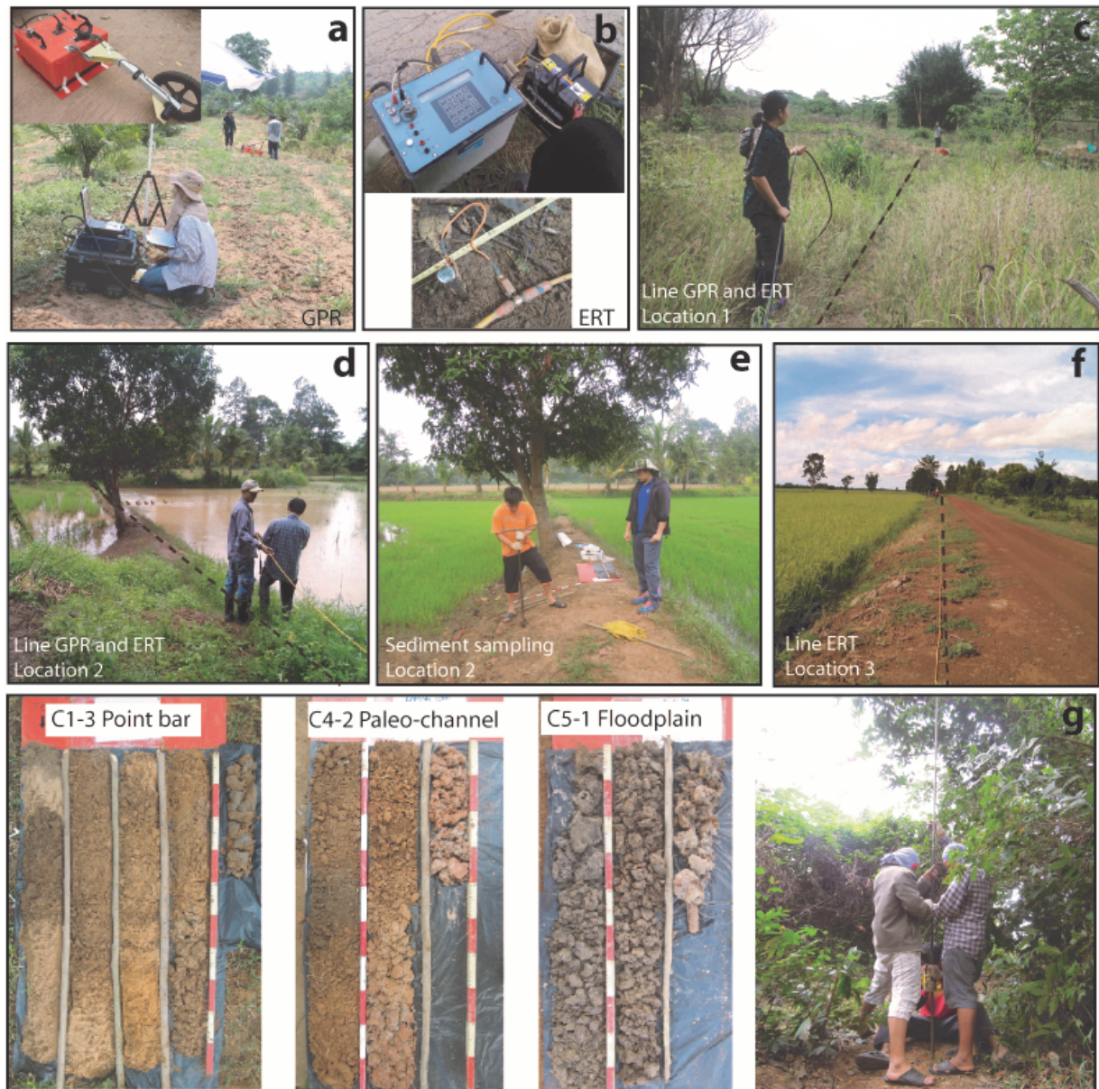
Figure 2: Photographs showing field investigation. (a) GPR survey using GSSI (SIR-20) instrument, (b) IRIS-SYSCAL R-1 Plus system of ERT survey, (c) line GPR and ERT survey from location 1, (d) ERT survey at location 2, (e) paleo-channel sediment from location 2 was drilled using hand auger, (f) longitudinal ERT line survey along the road at location 3, (g) sediment from three geomorphic units as point bar (C1-3 from location 1), paleo-channel (C4-2 from location 2) and floodplain (C5-1 from location).
