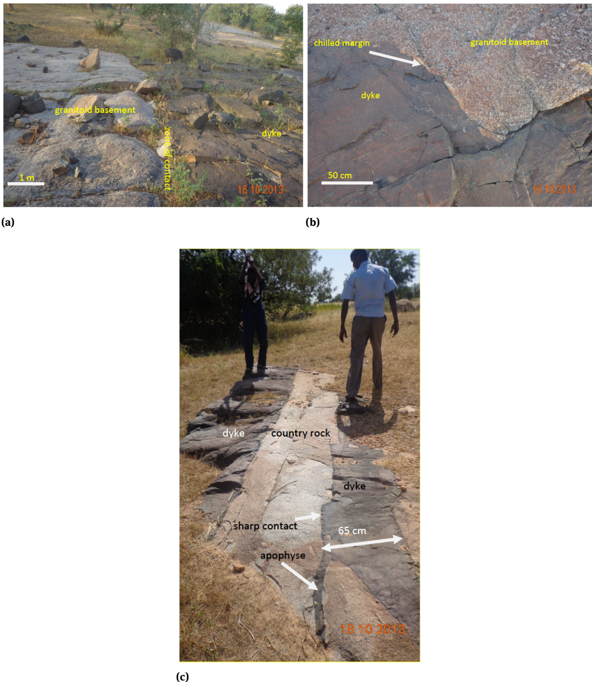
Figure 3: A: Sharp contact between granitoid wall-rock and Kilim dyke, B: Sharp contact between granitoid wall-rock and Kilim dyke showing a chilled margin. Increasing grain-size is obvious towards the dyke interior, C: Dyke edges with sharp contact between wall-rock and Barlo dyke.
