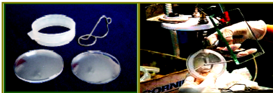
Fig. 10. Gasket, glass mould, clamp and filling unit of lenses.
