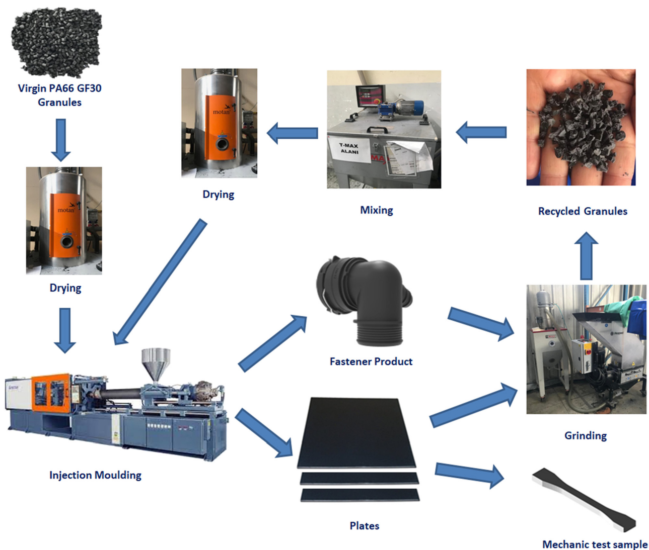
Scheme 1: Schematic representation of the mechanical recycling process of the PA66-GF30 composite.
