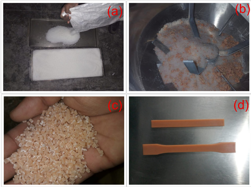
Figure 2: (a) HDPE granules, (b) blending of HDPE and TPW, (c) HDPE/TPW pellets, and (d) HDPE/TPW composite test specimens.
