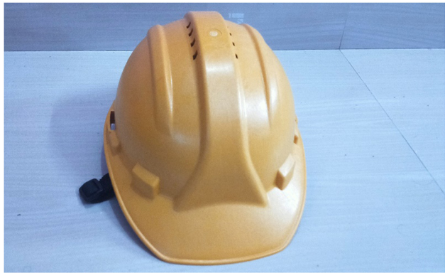
Figure 3: Fabricated helmet shell from HDPE/TPW composite in Concord Helmet & Safety Products Pvt. Ltd.
