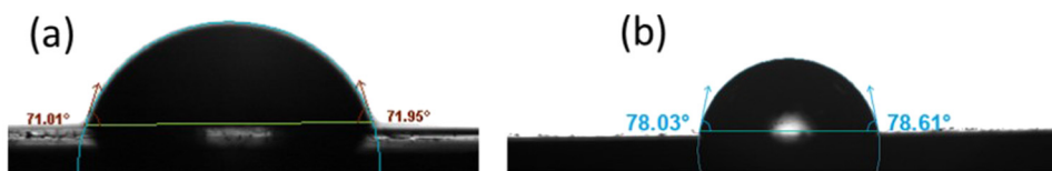
Figure 6: Contact angle of LPEA (a) and LPEA/0.5GO (b).
